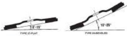
Individual flaps are designed to wear away evenly and present a constantly fresh working surface. They provide a cooler and more efficient grinding effect than conventional discs. No back up pads required. Best used for grinding and polishing metals, blending of welds and other metal finishing.
